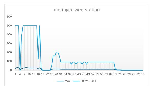
We then extracted the measurements during a specific period from the Aeroleaf® MWTs. A Modbus was installed on the boards where we log data such as the RPM and output in KW which can be visualized via a screen and an export.
