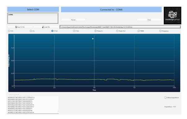
The measured data from 1 x Aeroleaf® MWT. We note that there was not much wind but this is still enough, together with the solar panels, to keep the battery at 70% (=3.22Kwh) and there are surpluses. The preliminary set parameters of the battery are 70 -> 73%.
